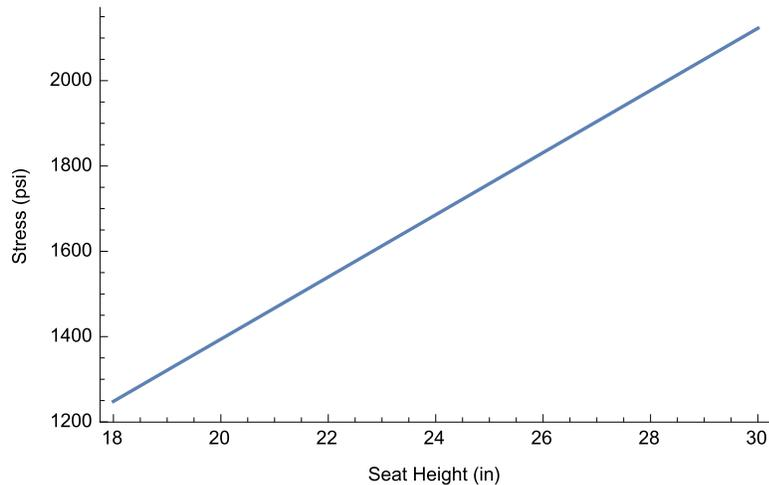
Figure 4: Stress at leg mortise for  $N = 3$ ,  $\theta = 17^\circ$ ,  $F_s = 200$  lb, and  $r = 1.125$  in.
