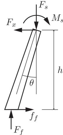
Figure 1: Free-body diagram of an idealized leg with no stretcher.
